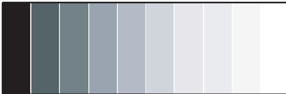
Figure 4-6. Typical Gray Bar Pattern for Adjusting Contrast
